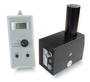
Fast count rates are achieved by using a YAP(Ce) scintillator, selected for its very fast (30 ns) decay time, and high speed electronics, designed to minimise dead-time. A plot of indicated counts against true counts is shown in section 6.
