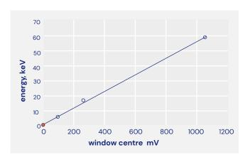
The coordinates of the three peak positions are transferred to a linear calibration curve relating X-ray energy to mV setting, as shown. Alternatively, the scale on the x axis in the above graph may be expressed in keV by using the calibration curve. The detector can then be used to generate the absolute energy spectrum of an unknown X-ray source by using the some procedure as for calibration.
