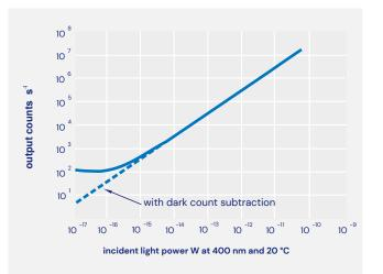
Typical counting sensitivity for DMO089C at 400 nm. Note that automatic dead time correction has been applied at high count rates. The dynamic range can be further extended at low count rates by dark count subtraction in the software.
