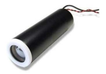
The signal lead is connected directly to the anode of the photomultiplier, allowing the freedom to work these modules into a range of electronic circuitry. The -HV is set by applying an external voltage, one-thousandth of the required voltage to the control input.
