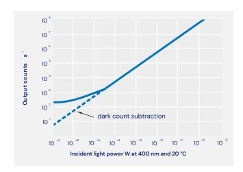
Typical counting sensitivity for P252USB at 400 nm. Note that automatic dead time correction has been applied at high count rates. The dynamic range can be further extended at low count rates by dark count subtraction by the user.
