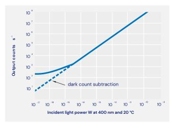
Typical counting sensitivity for P3OUSB at 400 nm. Note that automatic dead time correction has been applied at high count rates. The dynamic range can be further extended at low count rates by dark count subtraction by the user.
