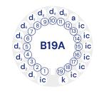
'ic' indicates an internal connection
